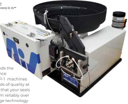
The ISP-1 machines feature a typical layout with a vibratory feeder bowl, gravity-fed track, and custom-designed installation tooling tailored to your unique part. ISP-1 machines deliver a quick, efficient, and precise process for installing O-rings and seals up to 1" OD into your parts.
